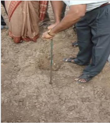
Drive the auger to a plough depth of 15 cm and draw the soil sample
